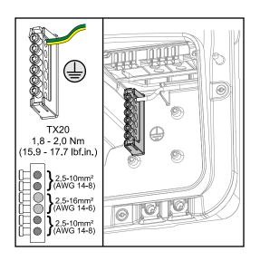
The ground electrode terminal ( Allows additional components to be earthed, such as:
