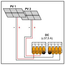
$PV 1 (I_{dcmax}) = 18.75 A / PV 2 (I_{dcmax}) = 18.75 A$
