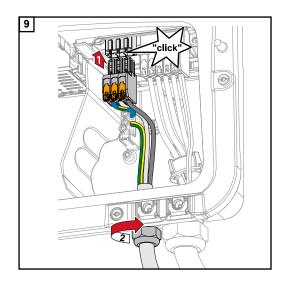
Insert the OP terminal into the OP slot until it engages. Tighten the union nut of the strain-relief device to the torque specified by the manufacturer.
