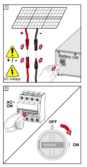
Connect the solar module strings (+/-). Switch on the battery connected to the inverter.
