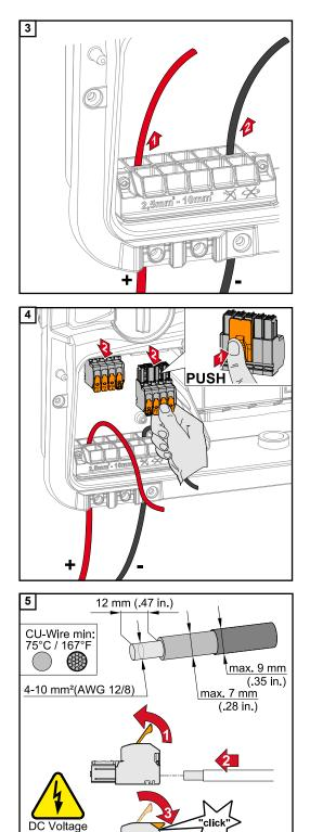
Select the cable cross section in accordance with the instructions in **Permitted cables** from page **45**.
