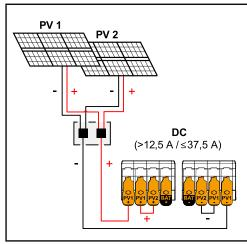
Combined solar module strings with total current (*I*dcmax) greater than 12.5 A.
