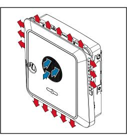
Ambient air is drawn in by the fan on the front side and blown out at the device sides. The even heat dissipation allows several inverters to be installed next to each other.
