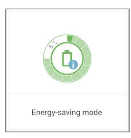
Energy saving mode is shown on the website of the inverter and in Solar.web by an "i" beside the battery symbol in the system overview.
