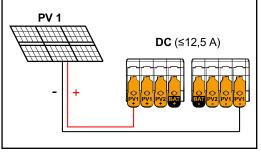
PV generator settings: PV 1: ON PV 2: OFF
