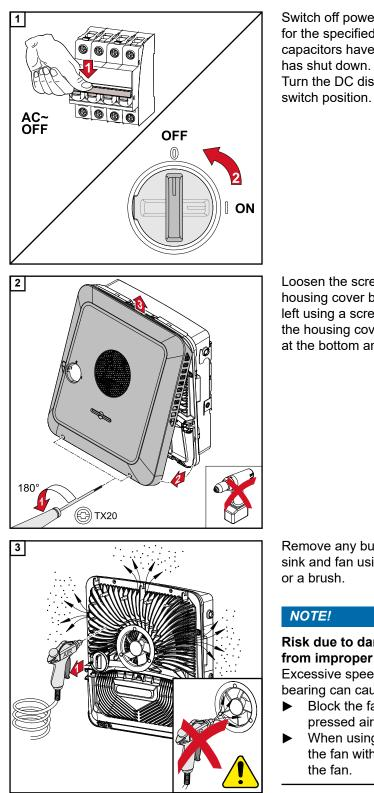
Switch off power to the inverter and wait for the specified time (2 minutes) until the capacitors have discharged and the fan has shut down. Turn the DC disconnector to the "Off"
