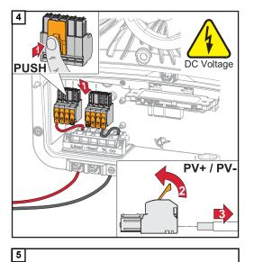
Remove the DC push-in terminals from the slots and disconnect them from the cables (only necessary if the installation already exists).
