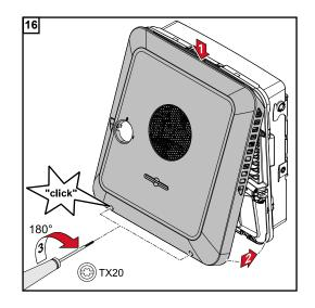
Clip the housing cover onto the inverter from above.
