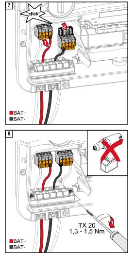
Insert the DC terminals into the respective slot until they engage.
