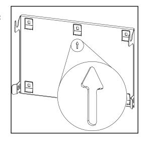
The separate mounting bracket (illustration) is also used as the gauge.
