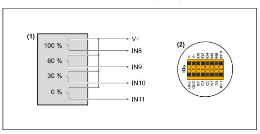
(1) Ripple control signal receiver with 4 relays, for effective power limitation.
