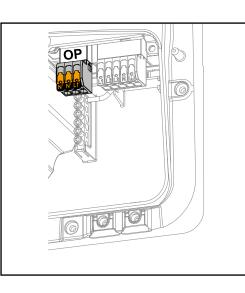
With the PV Point, in the event of a failure of the public grid, single-phase electrical devices can be connected to the Opportunity Power (OP) terminal and supplied with a maximum power of 3 kW, if enough power is available from the solar modules or an optional battery. In grid-connected operation, the OP terminal is not supplied with voltage, therefore the connected loads will not be supplied with power in this operating mode.
