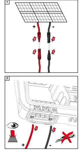
Push the DC cables through the DC bushings by hand.
