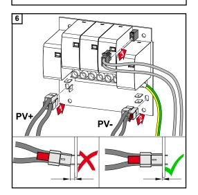
Connect the supplied cables to the respective connectors on the PC board.
