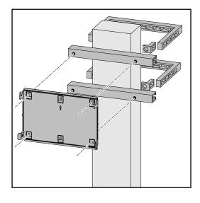
When installing the inverter on a mast or beam, Fronius recommends using the "Pole clamp" (order no. SZ 2584.000) mounting kit from Rittal GmbH.
