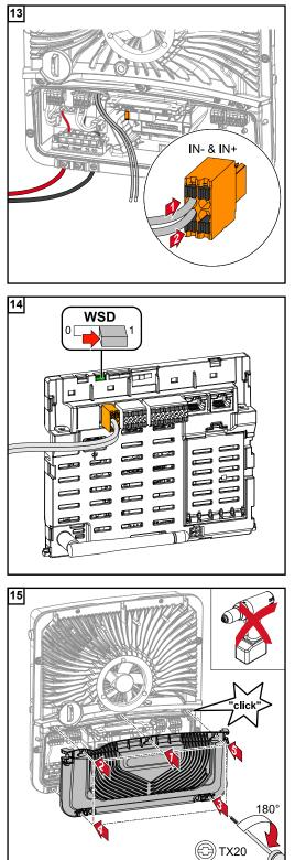
Connect the signal cable to the WSD push-in terminal on the IN- and IN+ slots, observing the labelling.
