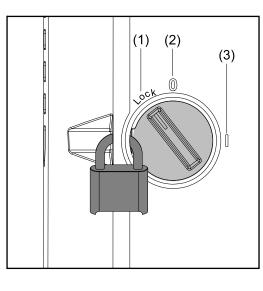
The DC disconnector has three switch settings:
