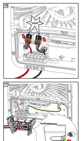
Push the DC push-in terminals into the corresponding slot until there is an audible click.
