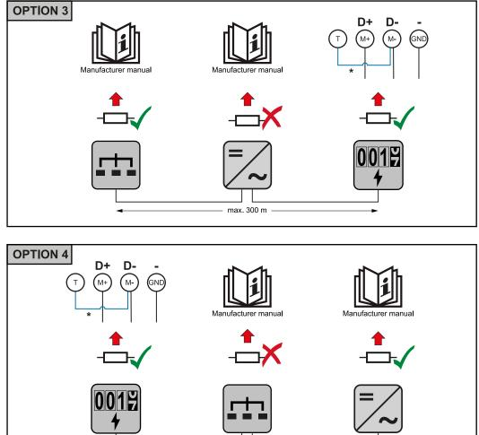
\* The terminating resistor is integrated in the Fronius Smart Meter TS and is manufactured with a bridge between the **M** and **T** connections (T = termination).
