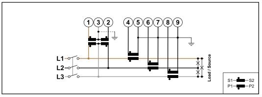
3 phases, 3 conductors (VT/CT connection)
