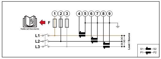
3 phases, 3 conductors (CT connection)
