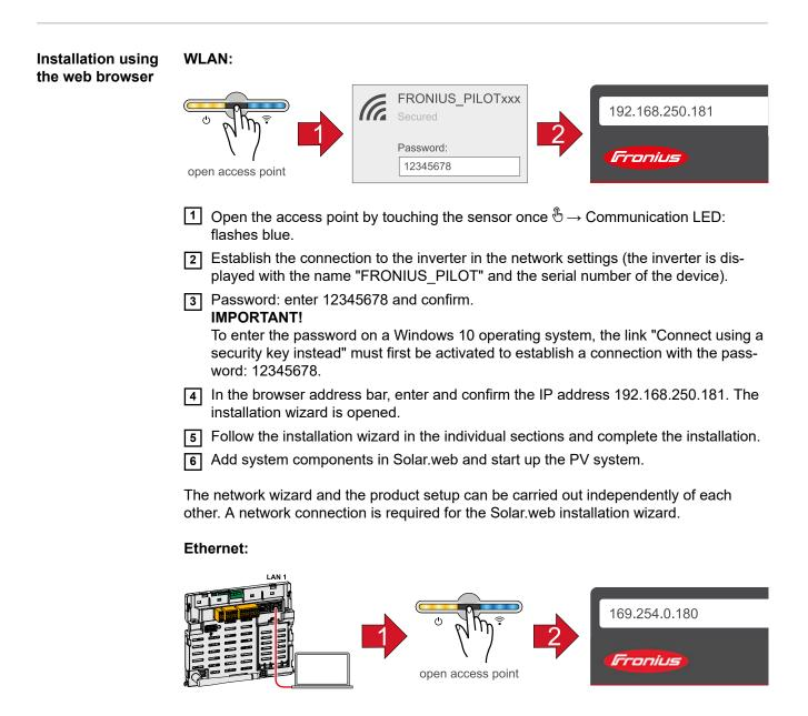
Establish a connection to the inverter (LAN1) with a network cable (CAT5 STP or higher).
