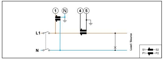
1 phase, 2 conductors (VT/CT connection)
