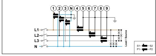
3 phases, 4 conductors (VT/CT connection)
