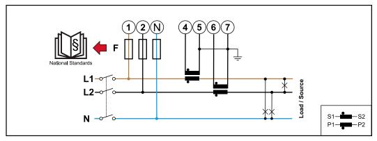
2 phases, 3 conductors (CT connection)
