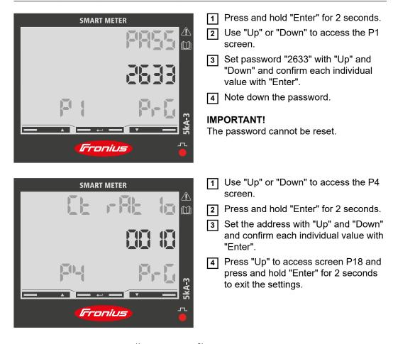
Ratio of current transformers<sup>1)</sup> (0001 -  $1000^{2}$ ). Ratio of voltage transformers<sup>1), 3)</sup> (001.0 -  $1000^{2}$ ).
