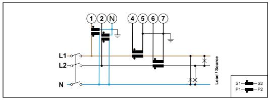
2 phases, 3 conductors (VT/CT connection)
