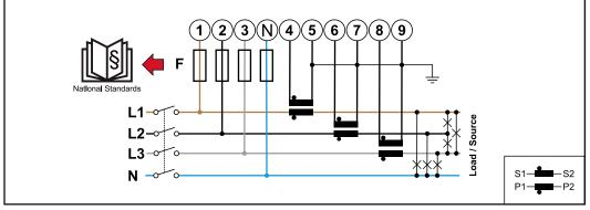
3 phases, 4 conductors (CT connection)
