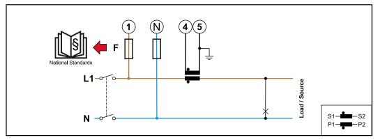
1 phase, 2 conductors (CT connection)
