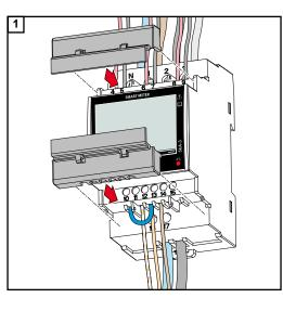
Insert the connection covers into the guides and press firmly.
