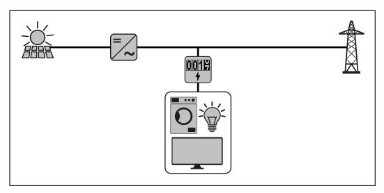
For use as a secondary meter to measure individual loads and producers, see chapter **Multi-meter system - Fronius SnaplNverter** on page **27**.
